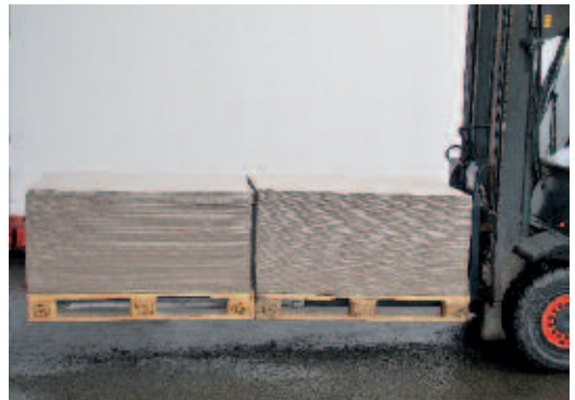
Handling of 2 pallets
